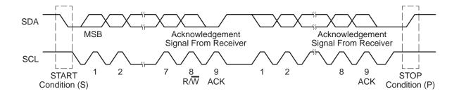
START and STOP conditions are generated by the master and are shown in Figure 15–3. A START condition is a high-to-low transition on the SDA line while SCL is high. A STOP condition is a low-to-high transition on the SDA line while SCL is high. The busy bit, I2CBB, is set after a START and cleared after a STOP.
